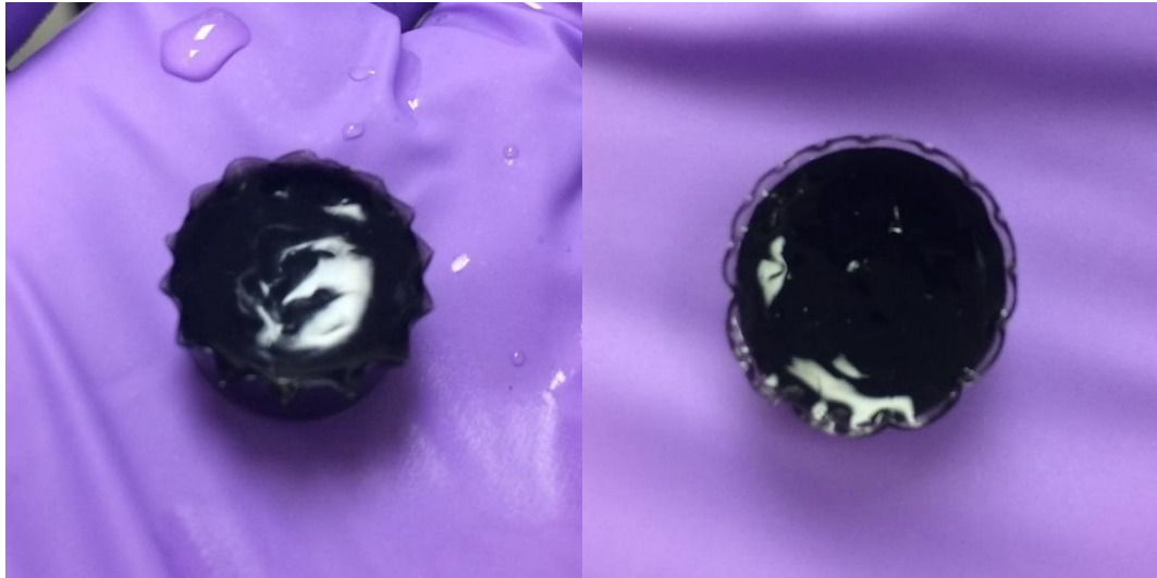
Figure 19. The wave-like edges on the top surface of hybrid gel samples were formed after gelation.
