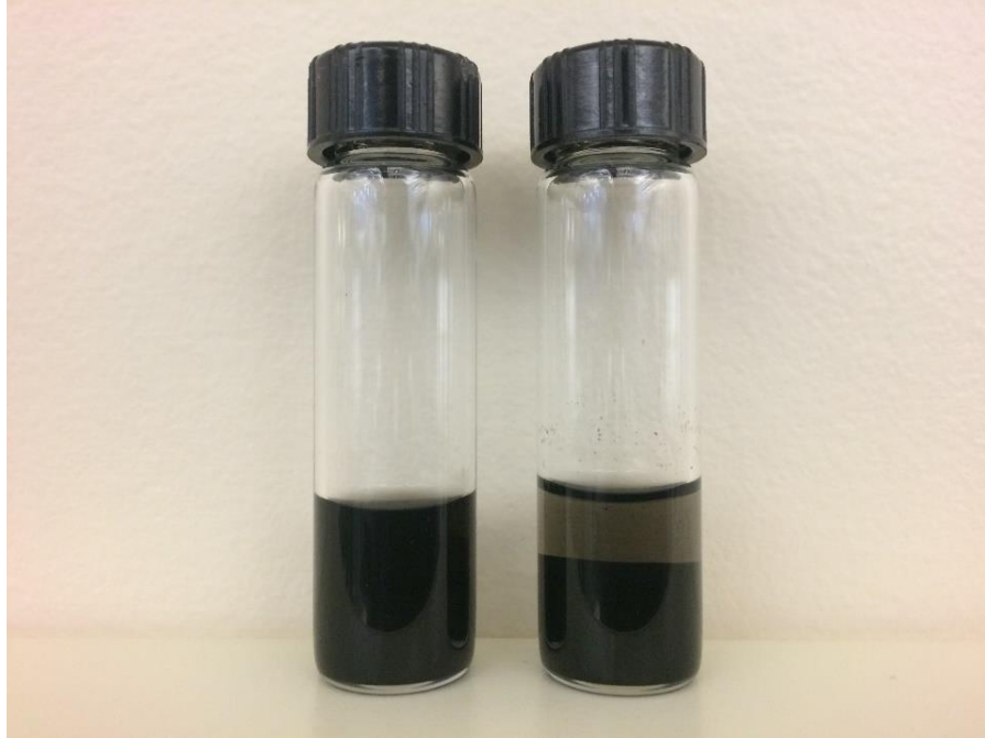
Figure 6. Two vials of 0.5 mg/ml dispersion of SWCNTs were put alone for two months. The left one was treated with sonication, centrifugation, and filtration. The right one was treated only by sonication.
