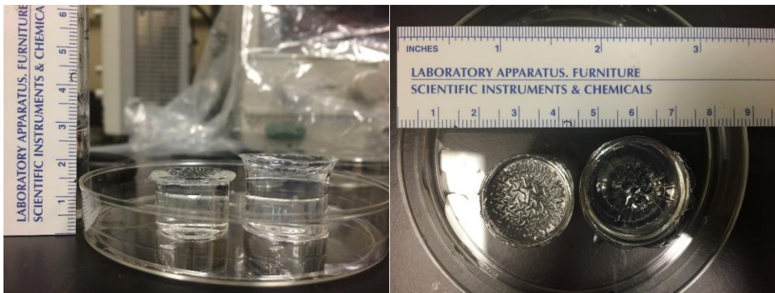
Figure 18. The surface patterns of PAAm gel samples with different dimensions.
