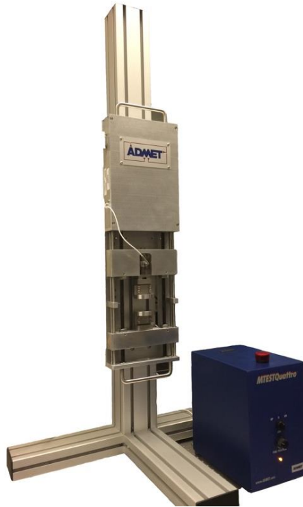
Figure 4. ADMET eXpert4000 universal testing machine with the MTESTQuattro materials testing system was used for the compression tests.
